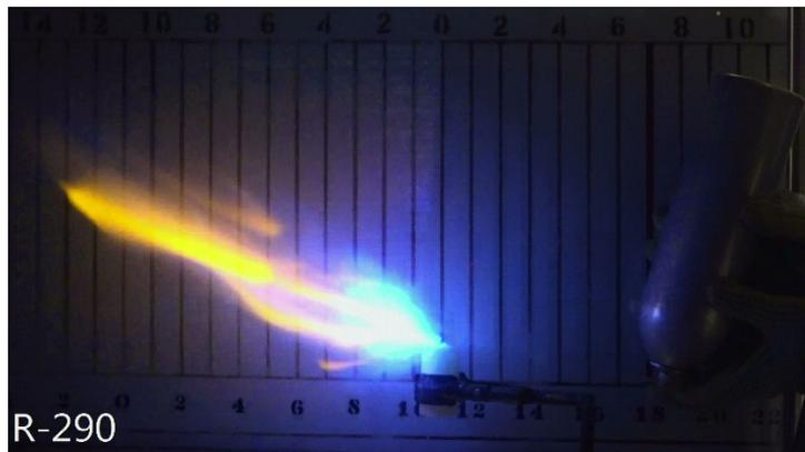
**Figure 2: Image of an R-290 Flame Projection Test Run**
