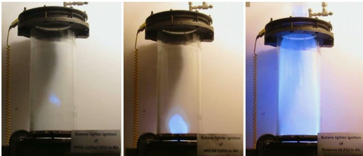
**Figure 4: Butane Lighter Tests @ 0.083 s Post-Ignition (R-1234yf [L], R-32 [C], R-290 [R])**
