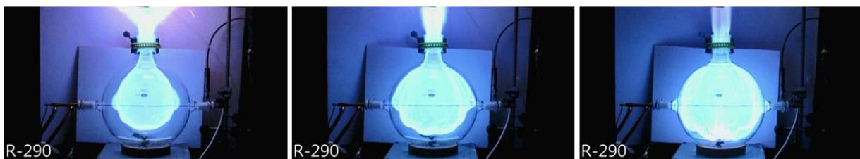
**Figure 3: Progressive Images of an R-290 Minimum Ignition Energy Test Run @ 1 mJ**
