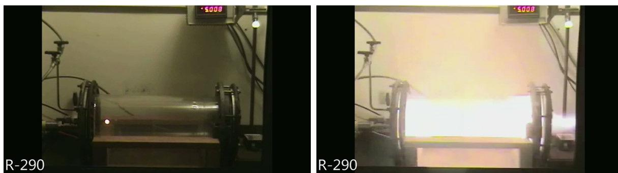
**Figure 5: Glow Wire Test with R-290 (Test Activation [L], 0.066 s from Initial Flame Front [R])**
