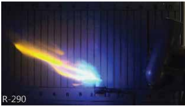
Figure 3: Image of an R-290 Flame Projection Test Run
